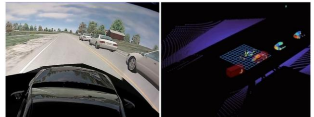
Figure 5: Co-simulation involving simulator cab, motion and visualization system (DSRI), simulated traffic and LIDAR sensor data (Chrono), object detection and LIDAR data visualized with Foxglove (ROS2).
