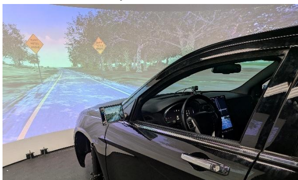
Figure 4: NADS-2 simulator with rendering for front and back views, side mirrors and backup camera used in multi driver interaction study alongside NADS-1 simulator.
