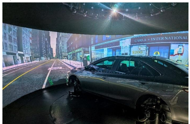
Figure 6: Co-simulation involving NADS-1 simulator cab, motion, vehicle dynamics and 360-degree visualization system alongside Carla.
