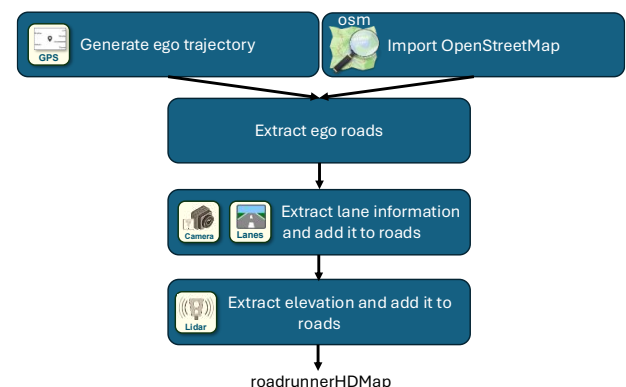
Figure 2 Workflow: Augment Standard Definition (SD) maps using recorded sensor data
