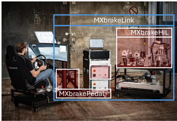
Figure 5 shows the different systems of the MXbrake environment with the MXbrakeLink, a combination of the standalone capable systems MXbrakeHiL and MXbrakePedal
