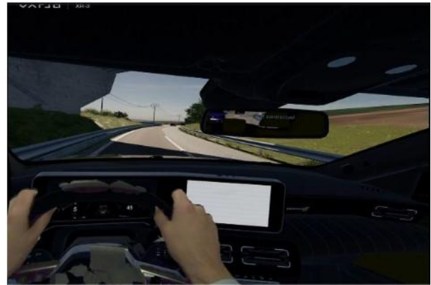
Figure 3: Display in the HMD with the Renault R5 cockpit, real hands and the virtual environment.
