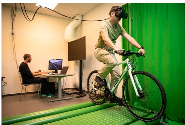
Figure 1: How We Roll: The VTI cycling simulator, featuring a free roller, a cyclist using a mixed reality headset, and the control computer in the background.
