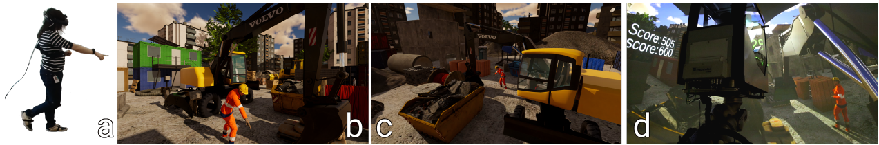
Figure 1: Communication setup and interfaces for the linked-lab experiment. The VR participant (a) controls the worker avatar (b) placed in the same virtual environment as the virtual construction machine (c), controlled from the interactive driving simulator (d).
