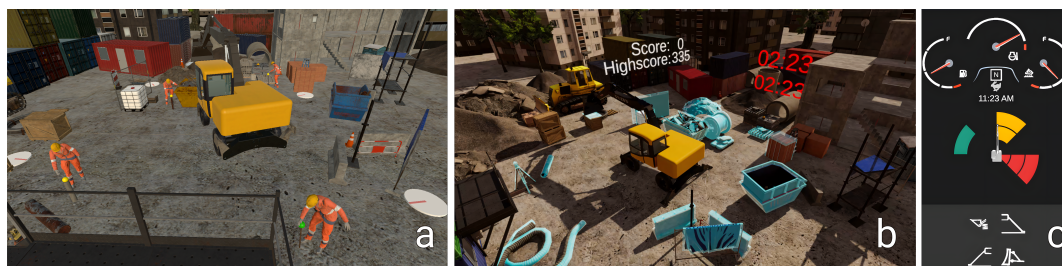
Figure 2: Participant Tasks. VR session task (a) starting positions and exemplary tasks for each sector. Excavator task (b) with task objects in turquoise, score, and time displays. Excavator cabin display (c), including assistance system (middle), colors indicate distance to detected worker.
