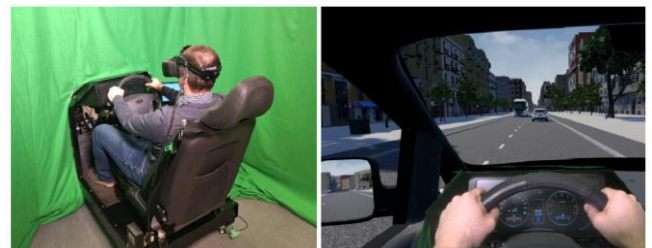
Figure 1. Fixed-base driving simulator used in the study, equipped with a vehicle mock-up and an XR headset.
